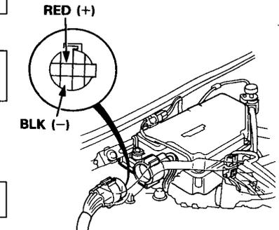
Check the self-diagnosis indicator. If OK, substitute a known-good control unit and retest. If symptom goes away, replace the original control unit.
