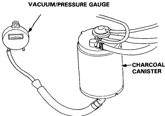
6. Place the shift or selector lever in 2nd gear or "2" range and raise the engine speed to 3,500 min<sup>-1</sup> (rpm). Vacuum should appear on the gauge within 1 minute.
