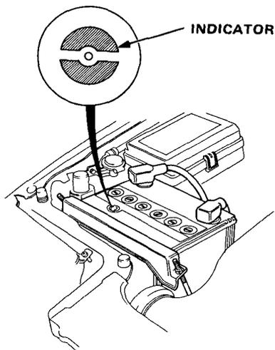
3. Test battery load capacity by connecting a battery tester, and applying a load of 3 times the battery ampere hour rating.
