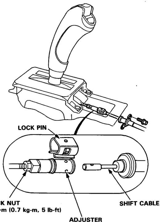
4. Check that the hole in the adjuster is perfectly aligned with the hole in the shift cable.
