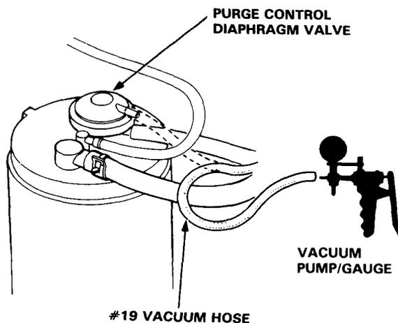
2. Start the engine and allow to idle.
