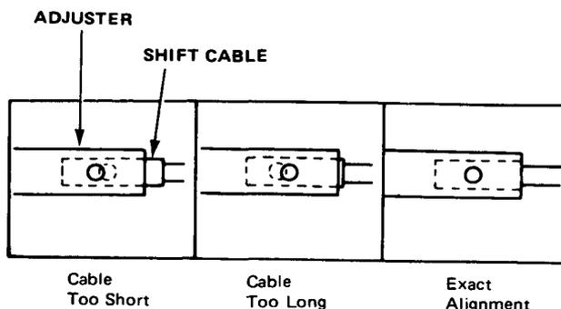
**NOTE:** There are two holes in the end of the shift cable. They are positioned 90° apart to allow cable adjustments in 1/4 turn increments.
