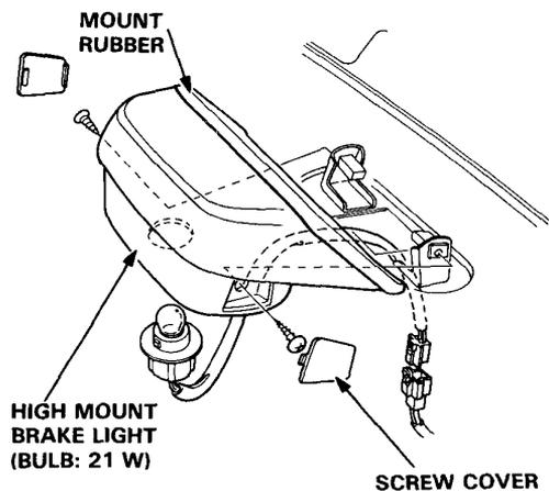
3. Turn the socket 45° counterclockwise to remove the bulb.
