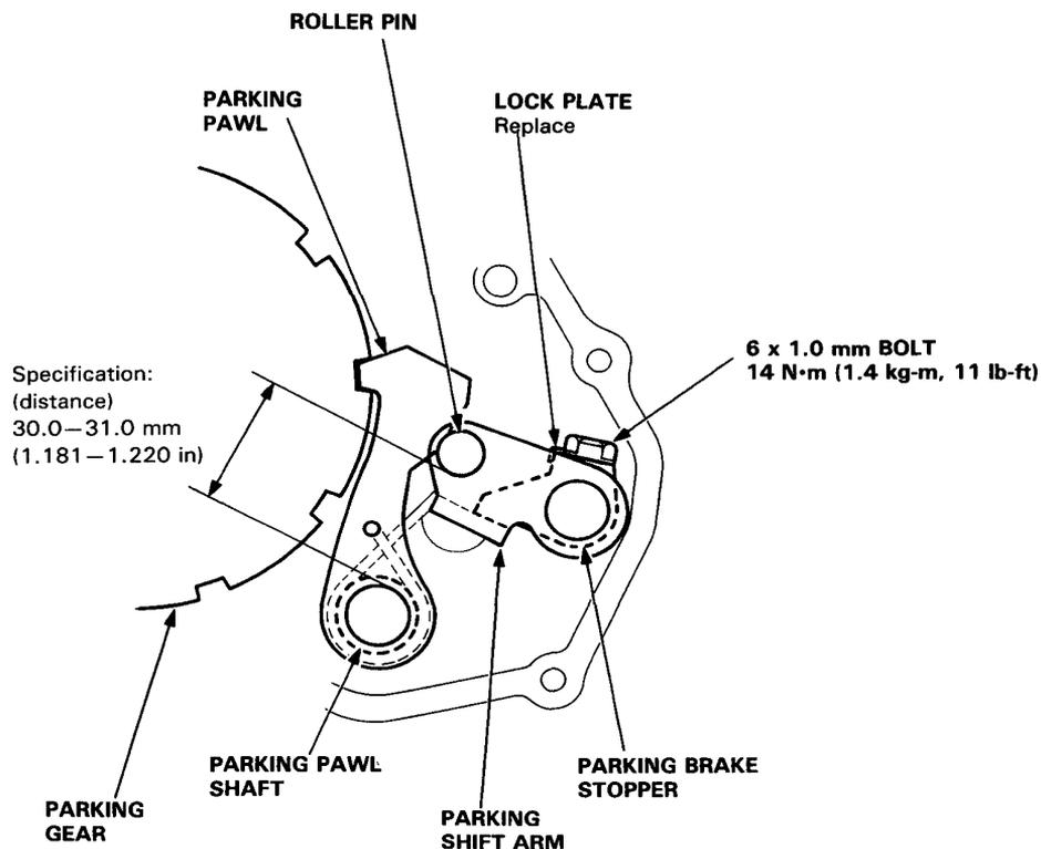
3. If the measurement is out of specification (distance), select the appropriate parking brake stopper using the table below, and install it on the parking shift arm.
