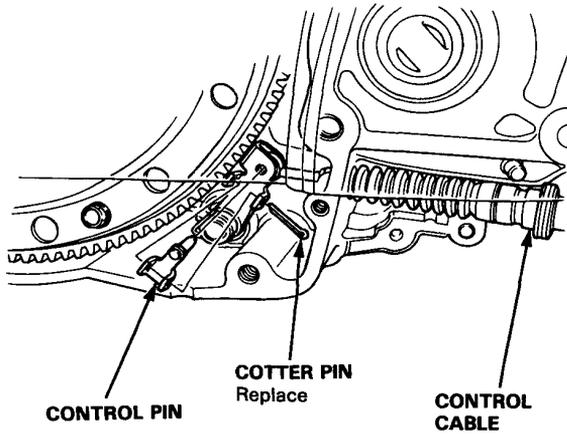
9. Pull the shift cable out of the by setting slot.
